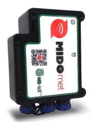
MiDoMet NBIoT Pressure is the specialized NBIoT datalogger for monitoring network pressure (or level) MiDoMeT NB-IoT is a self-powered universal device with extensive functionality. Through the 2 digital inputs it can be used to remotely read impulse meters, for billing purposes or to monitor the water network. Analog input can be used to collect data from 4-20mA or 0-5V sensor, like temp probe, pressure probe, level probe etc.
