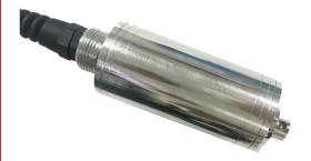
MiDoMet NTU1 is the simplest remote turbidity detection system. Turbidity measurement takes place through 90 ° NIR diffused light with nephelometric principle and with automatic temperature compensation.
